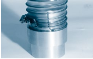
Variant 1: Expose the spiral, bend it to the inside and insert the conductive hose fitting.
