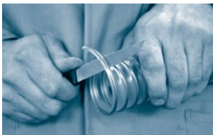
Step 1: Cut hose with a sharp knife along the steel wire.
