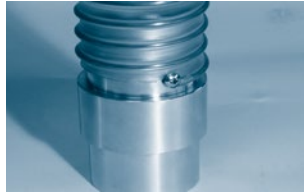
Variant 2: Expose the spiral and fix it, for example, by a rivet or screw.
