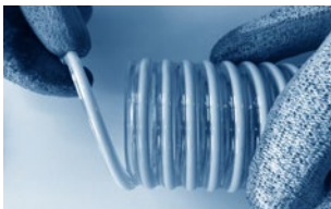
Step 2: Then, cut-off the protruding hard-plastic spiral with a side-cutter.
