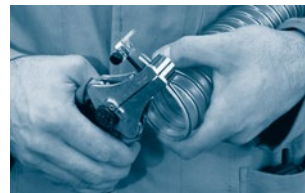
...or remove it more convenient with a precision insulation stripper.
