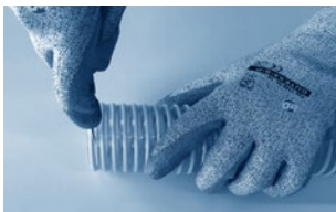
Step 1: Cut half of a circumference of the hose wall next to the grounding wire. The grounding wire stays on the residual part of the hose.
