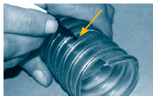
Mark the position of the bent wire.
