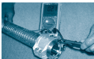
Check the correct contact between the adapters, by using an ohmmeter.
