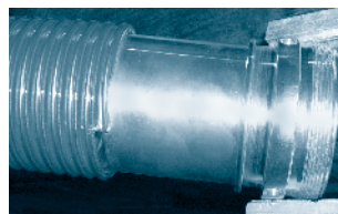
Pull the adapter over the hose, (anti-friction agent can be used if necessary).
