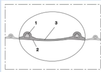
CNC machine hose for the woodworking industry, reinforced + for higher vacuum, highly flexible + compressible 4:1
