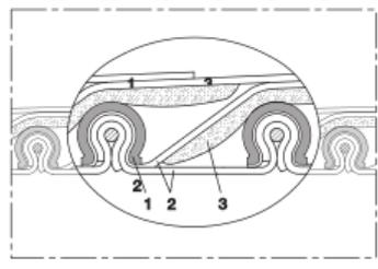
High-temperature hose, clamp profile hose (clip hose), multi-layer, insulating, suitable for slight overpressure (up to +1,292 °F)
