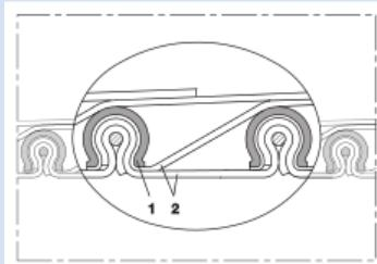
High-temperature hose, clamp profile hose (clip hose), multi-layer, insulating, suitable for slight overpressure (up to +1022°F)
