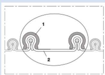
Electrically conductive clamp profile hose (clip hose), highly chemical resistant (up to +520°F)
