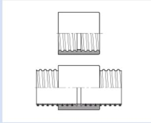
Spiral hose connector for connecting, lengthening or repairing spiral hoses, foodgrade
