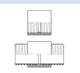
Spiral hose connector for connecting, lengthening or repairing spiral hoses, foodgrade
