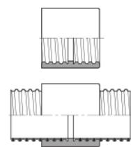
**Spiral hose connector for connecting, lengthening or repairing spiral hoses**
