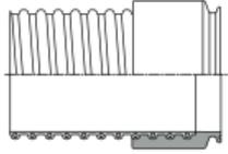
TRI-Clamp coupling to fit adapter acc. to DIN 32676, foodgrade
