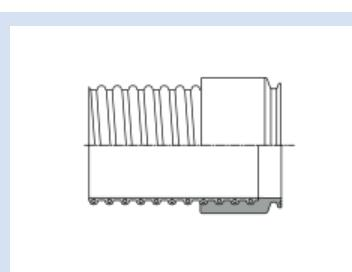
TRI-Clamp coupling to fit adapter acc. to DIN 32676, foodgrade
