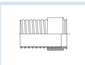
TRI-Clamp coupling to fit adapter acc. to DIN 32676
