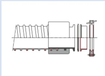
TRI clamp adapters based on DIN 32676 and ISO 2852
