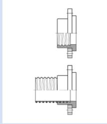
2-part loose flange to fit mating flanges acc. to DIN 2632/2633, hole pattern DIN-EN 1092-1, food safe
