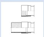
Flanged pipe according to the popular pipe systems in the ventilation field (for example Jacob-Standard), food-grade
