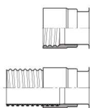
Flanged pipe according to the popular pipe systems in the ventilation field (for example Jacob-Standard), food-grade
