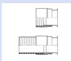
Flanged pipe according to the popular pipe systems in the ventilation field (for example Jacob-Standard)
