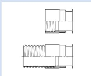
Flanged pipe according to the popular pipe systems in the ventilation field (for example Jacob-Standard)
