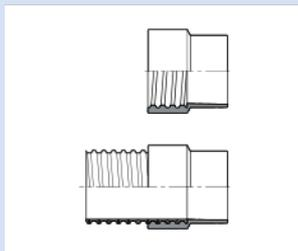
Soft sleeve to slide onto connectors or push into pipes, foodgrade
