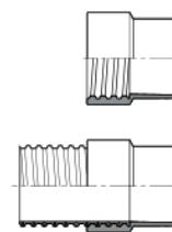
Soft sleeve to slide onto connectors or push into pipes
