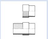
Soft sleeve to slide onto connectors or push into pipes
