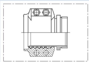
Special safety clamp coupling system for silos and dry-bulk transporters with couplers: Storz, Threaded connection, etc.
