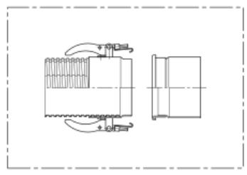
Connectors for connecting or attaching metal hoses
