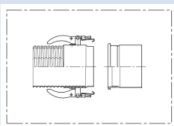
Connectors for connecting or attaching metal hoses
