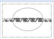
Abrasion-proof, oil resistant and polyurethane coated metal protection conduit; extremely robust and liquid tight; double folded metal profile
