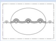
Abrasion-proof, oil resistant and robust polyurethane protection conduit; liquid tight; spiral: plastic coated spring steel wire
