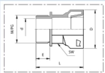
Plastic conduit connector; rigid connecting thread
