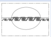
Abrasion-proof, oil resistant and polyurethane coated metal protection conduit; extremely robust and liquid tight; double folded metal profile
