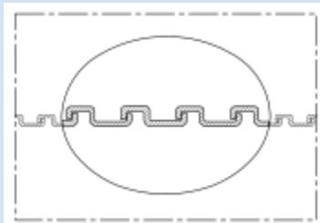
**Highly flexible metal protection conduit; robust; hooked metal profile**
